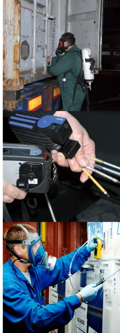
The container shown next was declared 'safe for entry' after measurements were taken between the seals of the doors. The photograph shows additional measurements being taken inside the cargo itself in order to be on the safe side.
