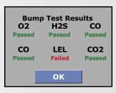
Color-coded text shows test or calibration results at a glance.
